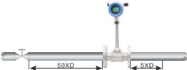
Regulating Valve, Half-open Gate Valve
