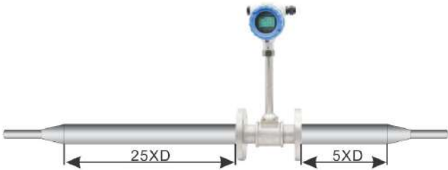
Concentric Expansion Pipeline
