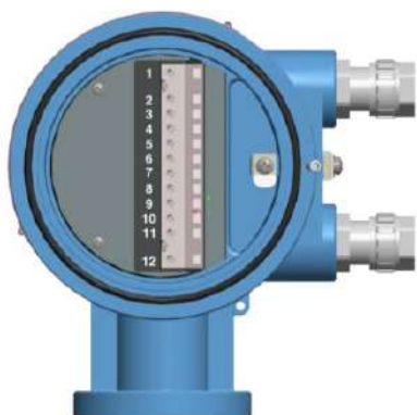
T1 transmitter terminal layout
